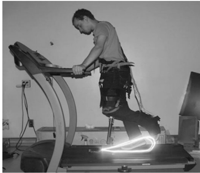
Fig. 6. The end-foot trajectory of a person, walking with the passive assistive walking device for a lower leg injury, developed at CSUF.
