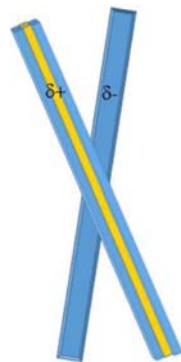
a) Attractive fiber-fiber interaction between b - and a -direction faces
