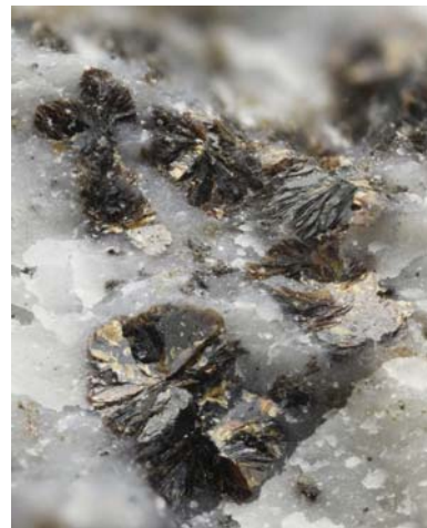
FIG. 1. Aggregates of radiating lath-shaped wicklundite crystals, showing typical very dark reddish brown colour and lustre. The fine-grained grey white matrix consists of manganiferous calcite. Field of view is 1.5 mm. Photo: Torbjörn Lorin.
