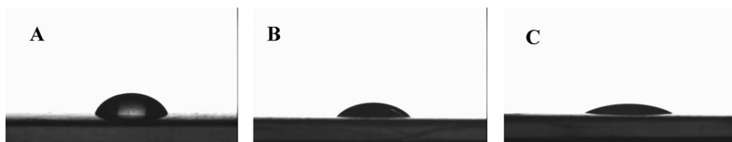
Figure 2. Contact angle of droplets. (A) 2,4-D-dimethylammonium salt, (B) 2,4-D 2-ethylhexyl ester, (C) HIL 3.
