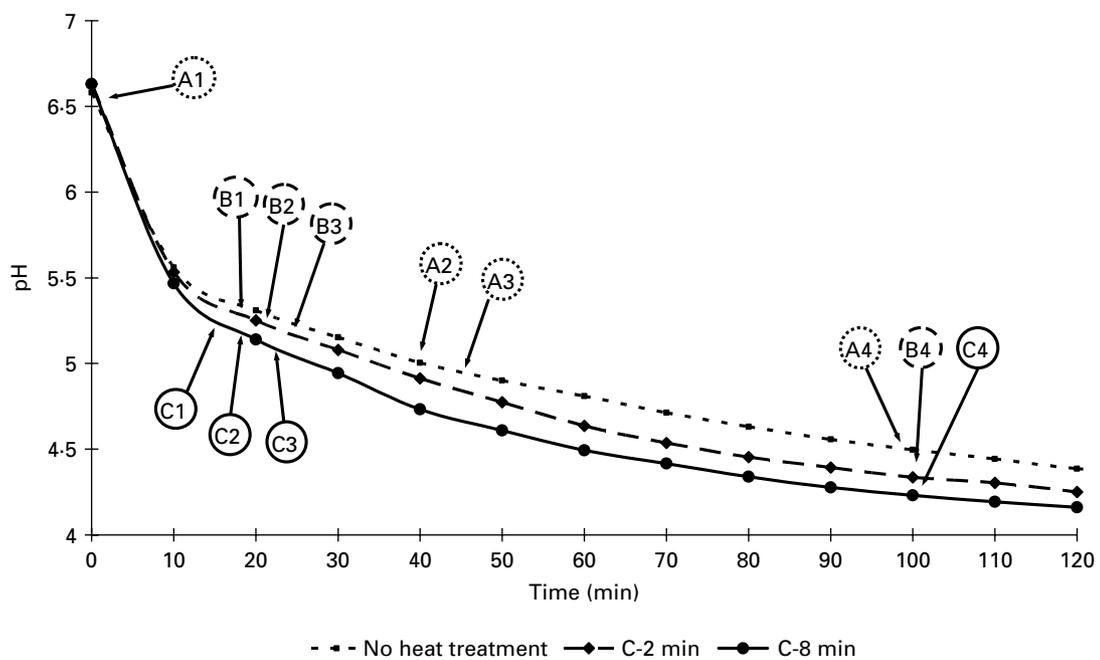
**Fig. 2.** Change in the pH profile of skim milk inoculated with glucono-delta-lactone (20 g/l) for (A) the control, (B) 90 °C-2 min and (C) 95 °C-8 min samples. The letters correspond to the confocal scanning laser microscopy images (Fig. 4).
