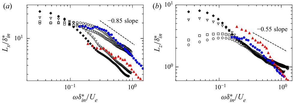
Figure 26. Normalised coherence lengths for ZPG locations ( $\circ$ ,  $x/c = -0.60$ , and  $\square$ ,  $x/c = -0.47$ ) and APG locations ( $\nabla$ ,  $x/c = -0.14$ , and  $\+$ ,  $x/c = -0.08$ ) in (a) streamwise and (b) spanwise directions:  $\bullet$  (blue), ZPG data by Hu (2021) at  $Re_\theta = 4889$ ;  $\blacktriangle$  (red), APG data by Hu (2021) at  $Re_\theta = 8670$ .
