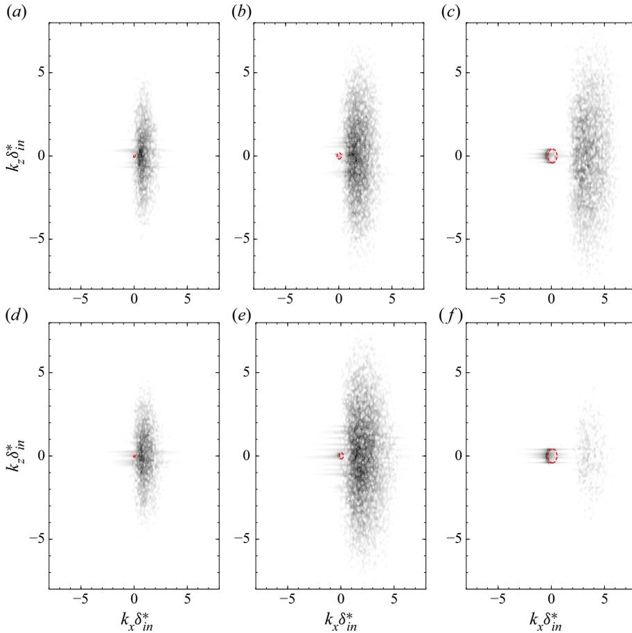
Figure 30. Normalised 2D wavenumber-frequency spectra  $\overline{\Psi}_{pp}(\mathbf{k}; \omega) = \Psi_{pp}(\mathbf{k}; \omega)(U_\infty/\tau_w^2 \delta_{in}^{*3})$  measured at three dimensionless frequencies: (a,d)  $\omega\delta_{in}^*/U_\infty = 0.34$ ; (b,e)  $\omega\delta_{in}^*/U_\infty = 0.76$ ; (c,f)  $\omega\delta_{in}^*/U_\infty = 1.73$ . APG locations: (a–c)  $x/c = -0.14$ ; (d–f)  $x/c = -0.08$ . Trace of the acoustic domain (red dashed line) (Cohen & Gloerfelt 2018).
