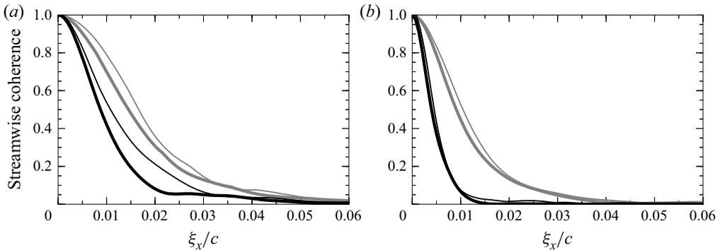
Figure 22. Coherence functions,  $\gamma^2$ , at various streamwise separations on the aerofoil suction side: (a) 1600 Hz and (b) 5000 Hz. ZPG locations  $x/c = -0.60$  (thin grey line) and  $x/c = -0.47$  (thick grey line); APG locations  $x/c = -0.14$  (thin black line) and  $x/c = -0.08$  (thick black line).
