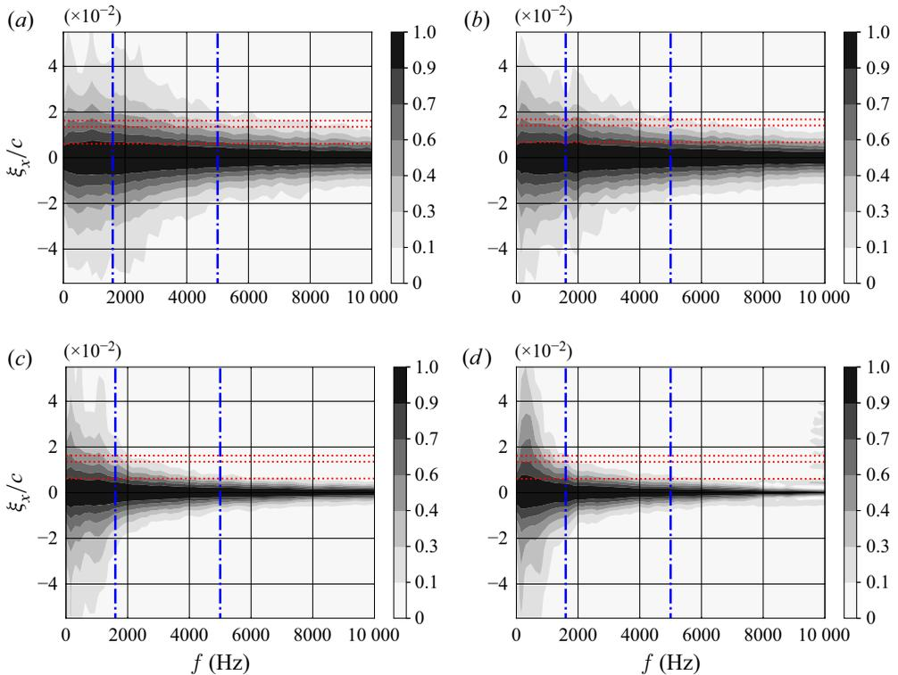
Figure 18. Contours of streamwise coherence of fluctuating pressure for ZPG and APG regions: (a)  $x/c = -0.60$ ; (b)  $x/c = -0.47$ ; (c)  $x/c = -0.14$ ; and (d)  $x/c = -0.08$ . Symbols:  $\cdots$  (red) spatial separations  $\xi_x/c = 0.007, 0.013, 0.016$  used in figures 20 and 21;  $-\cdot-$  (blue) frequencies of 1600 and 5000 Hz used in figure 22 and 23.
