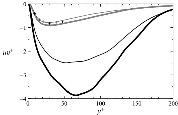
Figure 10. Reynolds stress component normalised with inner scale along wall-normal direction: ZPG locations  $x/c = -0.60$  (thin grey line) and  $x/c = -0.47$  (thick grey line); APG locations  $x/c = -0.14$  (thin black line),  $x/c = -0.08$  (thick black line); +, ZPG data by Spalart (1988) with  $Re_\theta = 300$ .
