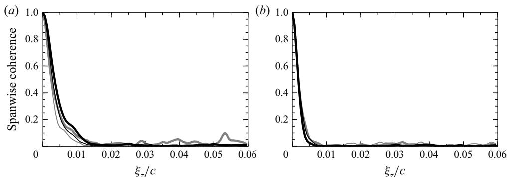
Figure 23. Coherence functions,  $\gamma^2$ , at various spanwise separations on the aerofoil suction side: (a) 1600 Hz and (b) 5000 Hz. ZPG locations  $x/c = -0.60$  (thin grey line) and  $x/c = -0.47$  (thick grey line); APG locations  $x/c = -0.14$  (thin black line) and  $x/c = -0.08$  (thick black line).
