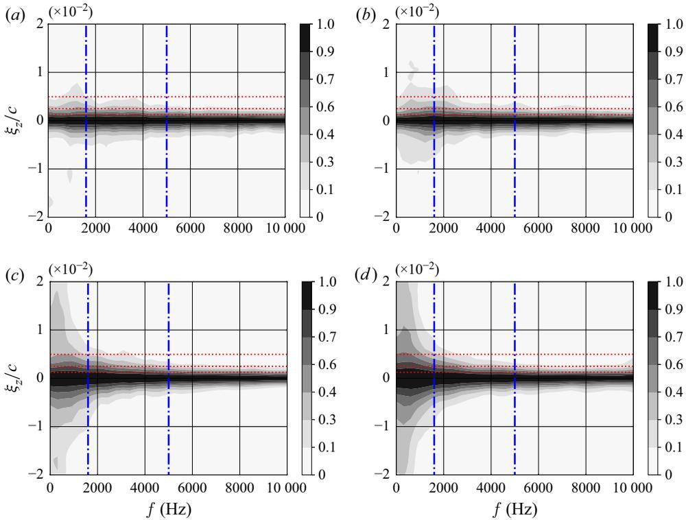
Figure 19. Contours of spanwise coherence of fluctuating pressure for ZPG and APG regions: (a)  $x/c = -0.60$ ; (b)  $x/c = -0.47$ ; (c)  $x/c = -0.14$ ; and (d)  $x/c = -0.08$ . Symbols:  $\cdots$  (red), spatial separations  $\xi_z/c = 0.0019, 0.0025, 0.0049$  used in figures 20 and 21;  $-\cdot-$  (blue) frequencies 1600 and 5000 Hz used in figures 22 and 23.
