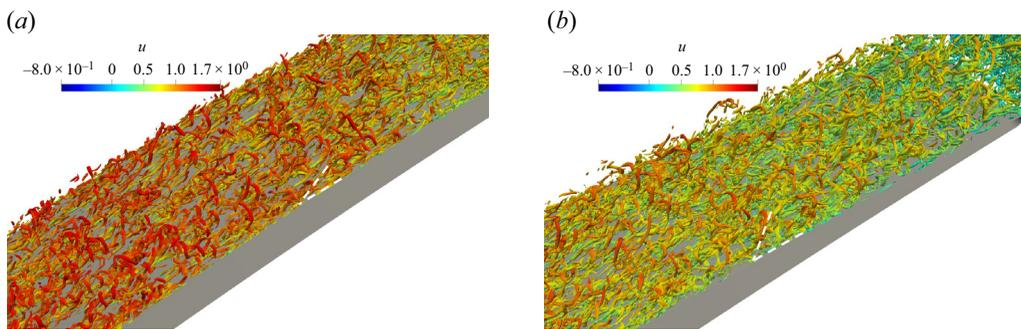
Figure 11. Swirling strength criterion (Zhou *et al.* 1999; Wu *et al.* 2017) isocontours coloured by streamwise velocity component by Wu *et al.* (2019): (a) ZPG portion (mid-chord) and (b) APG (or TE) portion.
