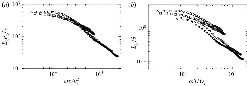
Figure 27. Normalised streamwise coherence lengths for ZPG locations ( $\circ$ ,  $x/c = -0.60$ , and  $\square$ ,  $x/c = -0.47$ ) and APG locations ( $\nabla$ ,  $x/c = -0.14$ , and  $\blackplus$ ,  $x/c = -0.08$ ) in (a) inner and (b) outer variable scalings.
