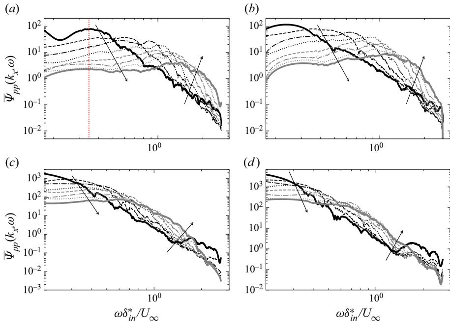
Figure 31. Normalised 2D wavenumber-frequency spectra as function of frequency at increasing  $k_x \delta_{in}^*$ .  $k_x \delta_{in}^* = 0.36$  (solid black line) to  $k_x \delta_{in}^* = 2.11$  (solid thick grey line), with increments of 0.25: (a)  $x/c = -0.60$ ; (b)  $x/c = -0.47$ ; (c)  $x/c = -0.14$ ; and (d)  $x/c = -0.08$ .
