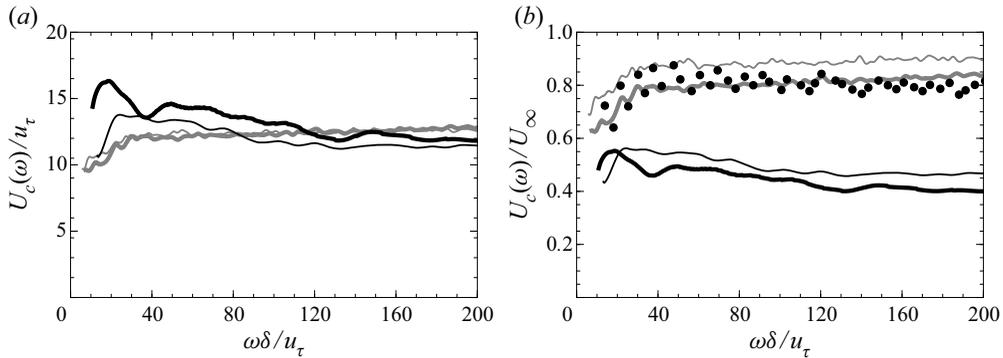
Figure 32. Normalised convection velocities as function of dimensionless frequency at four locations on the aerofoil suction side: ZPG locations  $x/c = -0.60$  (thin grey line) and  $x/c = -0.47$  (thick grey line); APG locations  $x/c = -0.14$  (thin black line) and  $x/c = -0.08$  (thick black line); •, data by Choi & Moin (1990); (a) inner variables scaling; (b) outer variables scaling.
