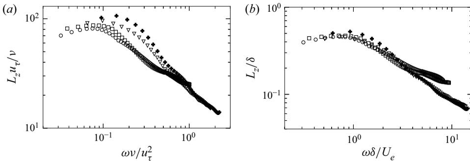
Figure 28. Normalised spanwise coherence lengths for ZPG locations ( $\circ$ ,  $x/c = -0.60$ , and  $\square$ ,  $x/c = -0.47$ ) and APG locations ( $\nabla$ ,  $x/c = -0.14$ , and  $\blackplus$ ,  $x/c = -0.08$ ) in (a) inner and (b) outer variable scalings.
