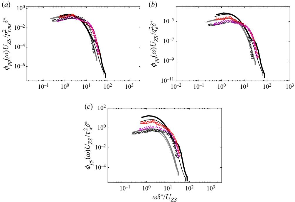
Figure 14. Spanwise-averaged wall-pressure spectra at four locations on the aerofoil suction side scaled with Zaragola–Smits scaling,  $U_{ZS} = U_e \delta^* / \delta$ : ZPG locations  $x/c = -0.60$  (thin grey line) and  $x/c = -0.47$  (thick grey line); APG locations  $x/c = -0.14$  (thin black line),  $x/c = -0.08$  (thick black line);  $\Delta$ , ZPG (black), APGs (red), APGw (magenta) data by Cohen & Gloerfelt (2018). (a,b) Outer and (c) mixed inner–outer variables scaling.
