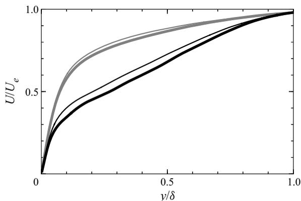
Figure 4. Dimensionless velocity profiles: ZPG locations  $x/c = -0.60$  (thin grey line) and  $x/c = -0.47$  (thick grey line); APG locations  $x/c = -0.14$  (thin black line),  $x/c = -0.08$  (thick black line).
