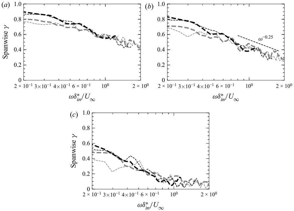
Figure 21. Spanwise  $\gamma(\xi_z, \omega)$  frequency distribution for different spatial separations at four location on the aerofoil suction side: (a)  $\xi_z/c = 0.0019$ ; (b)  $\xi_z/c = 0.0025$ ; (c)  $\xi_z/c = 0.0049$ . ZPG locations  $x/c = -0.60$  (thin grey line) and  $x/c = -0.47$  (thick grey line); APG locations  $x/c = -0.14$  (thin black line),  $x/c = -0.08$  (thick black line).
