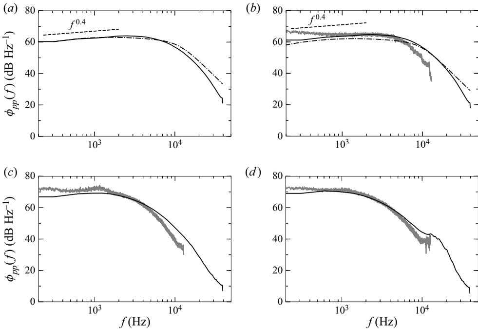
Figure 12. Spanwise-averaged wall-pressure spectra at four locations on the aerofoil suction side: —, DNS-NS; - - -, Goody's model, and — (grey), UdeS measurements; (a)  $x/c = -0.60$ , (b)  $x/c = -0.47$ , (c)  $x/c = -0.14$  and (d)  $x/c = -0.08$ .
