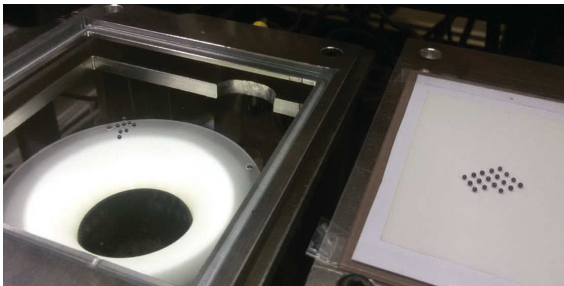
Fig. 7. Calibration of the second camera. On the left, area1 used as a gripping area seen by the first camera; on the right, virtual grid under construction in area2.
