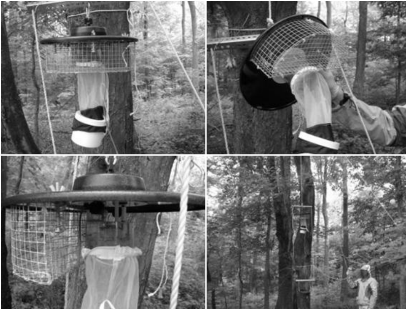
Fig. 1. Photographs of a modified CDC miniature light trap (with CO 2 and light sources removed) with a small wire cage used to hold either a guinea-pig or chicken as a mosquito attractant.
