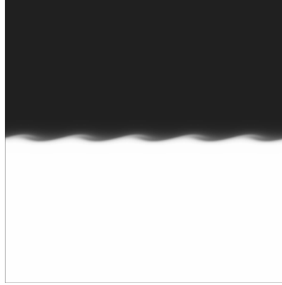
FIGURE 28. Snapshot of the density field at time t = 5 s from the time-evolution simulation of a parallel shear constructed with the density and horizontal velocity profile from the maximum displacement of the wave of amplitude a/h_1 = 1.51 , perturbed with an unstable normal mode of wavenumber k = 77\pi/5 \approx 0.4 \text{ cm}^{-1} . The computational domain is of 77 \text{ cm} \times 77 \text{ cm} , periodic boundary conditions in the horizontal direction, while the resolution is of 1024 points in the vertical.
