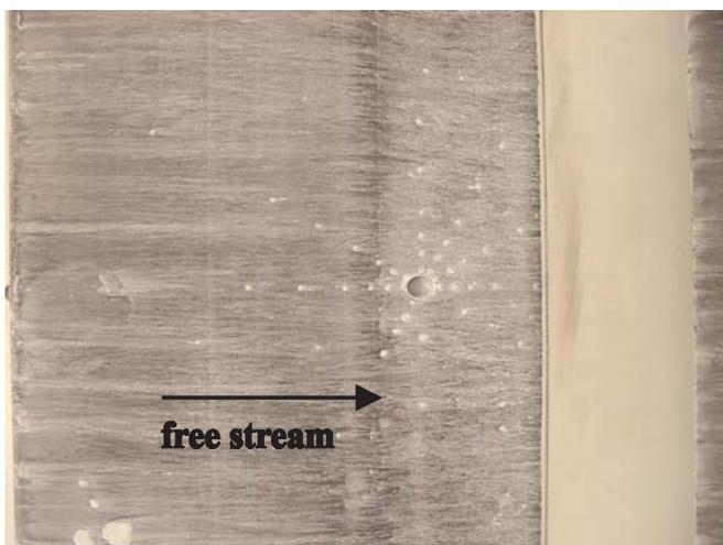
Figure 14. Oil flow on car body, exhaust-off.
