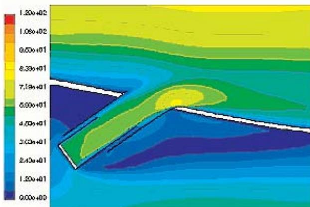
Figure 18(c). Velocity contours around the exhaust area at 100% overlap.
