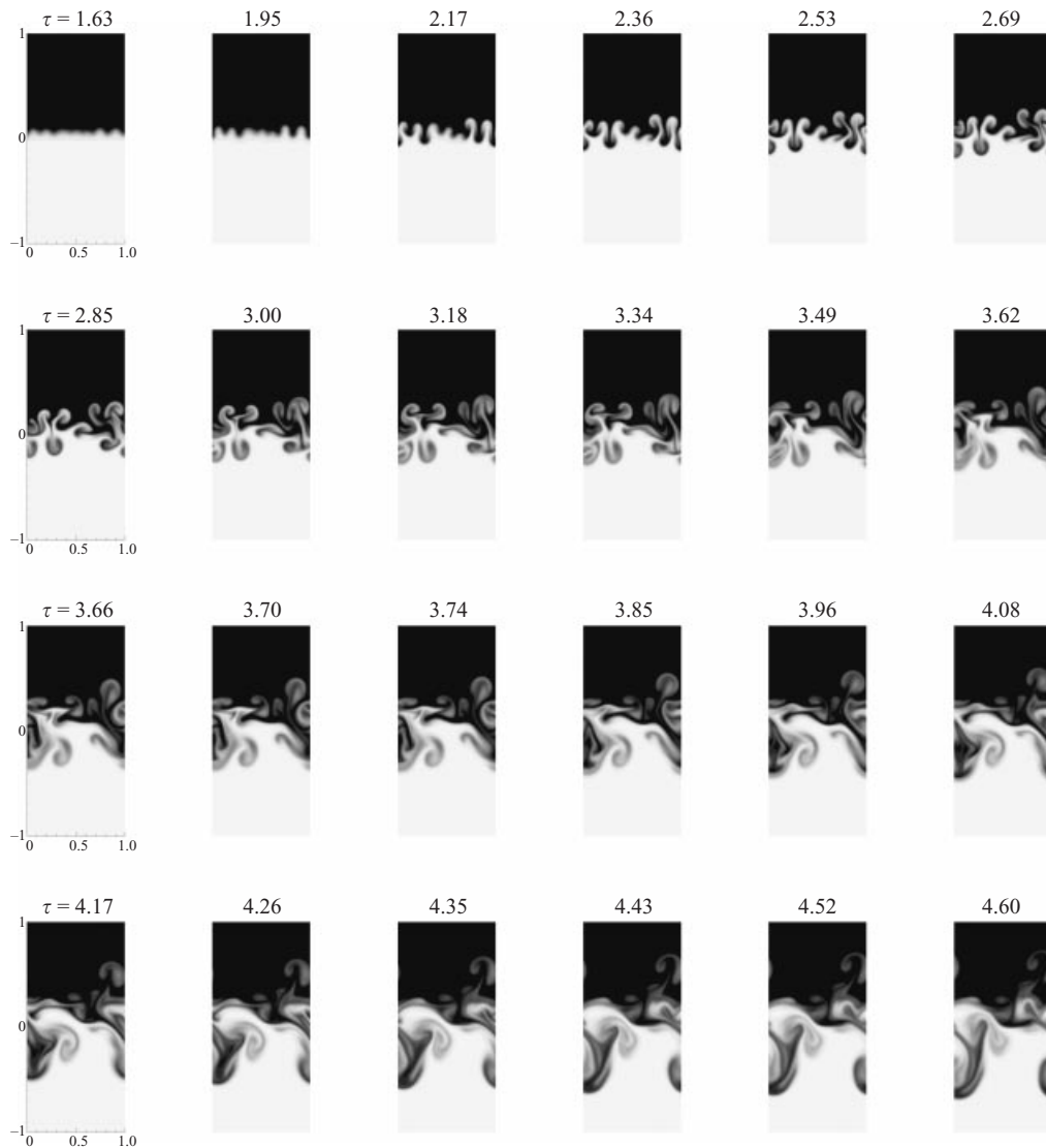
FIGURE 3. Time series of the temperature field in a 1(x) by 2(z) box from the two-dimensional simulations. The interface between cold (black) and warm (white) fluids is perturbed by the \delta T(x, y = 0) slice taken from the spatially random disturbances in the three-dimensional simulations.
