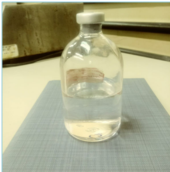
Figure 1 An inert headspace performed in a 120-mL bottle, using 50–60 mL of seawater to CO 2 extraction.
