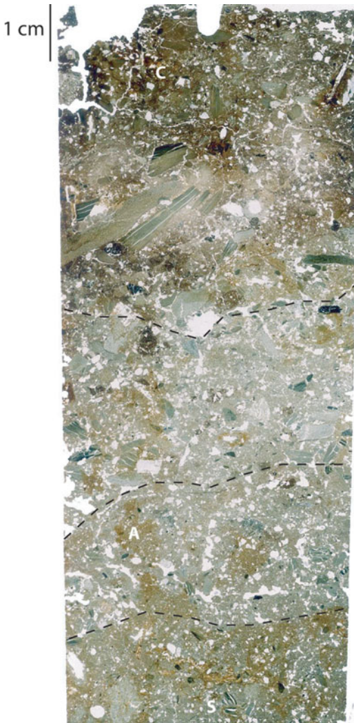
Figure 8. Microstratigraphy of terrace wall (thin-section micromorphology): shaped clumps showing successive applications; diversity of materials: clayey silt sediments from occupation layers (S), clayey materials from the marshes (A) or burnt mud waste (C) (image © Julia Watez).
