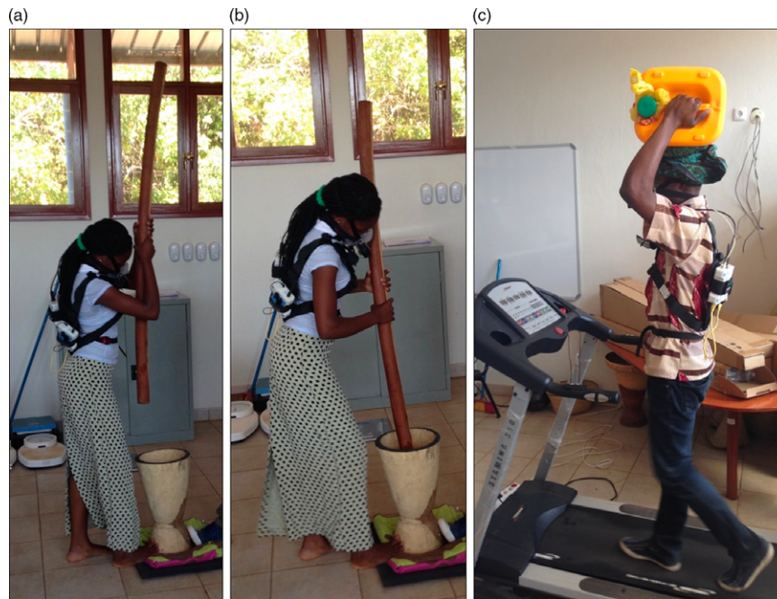
Fig. 2 (colour online) (a and b) Study participant uses a traditional pilão by repeatedly raising the long wooden pestle above her head and striking it down into the large wooden mortar. (c) Study participant walks on treadmill with 20 litres of water (20.5 kg, including container) loaded on her head. Photo Credit: Kory Russel
