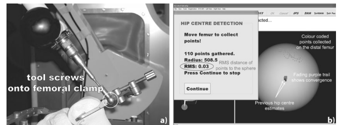
Fig. 8. (a) Cutter insert used to generate a set of measurements for the distal femur location during hip centre estimation and (b) the intra-operative GUI used during the hip centre estimation process.
