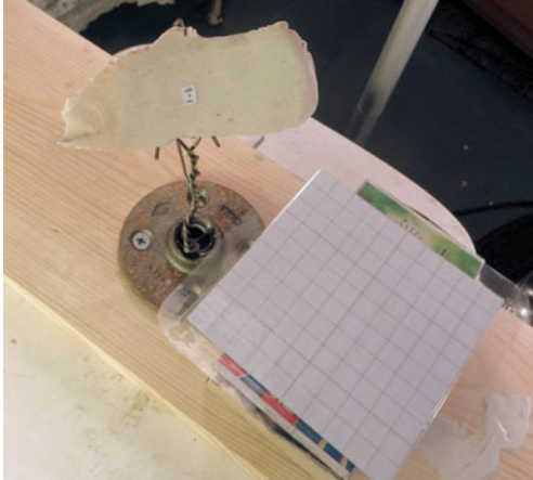
Figure 3. Expedient setup: objects are placed on a wire stand, and images are taken as the photographer moves around the object.
