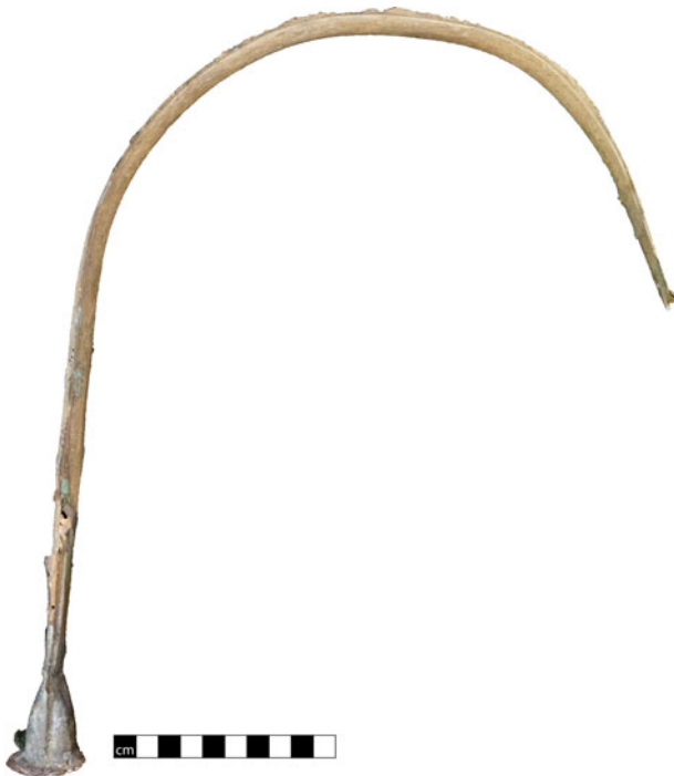
Fig. 11. An as-cast replica sword bent into a U-shape
