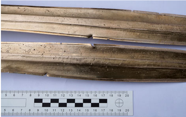
Fig. 6. Notches caused by edge-on-edge contact between the replica swords (Sword 2.1 above, Sword 2.2 below)
