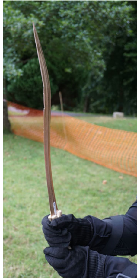
Fig. 8. Sword 2.2 bent in both directions
