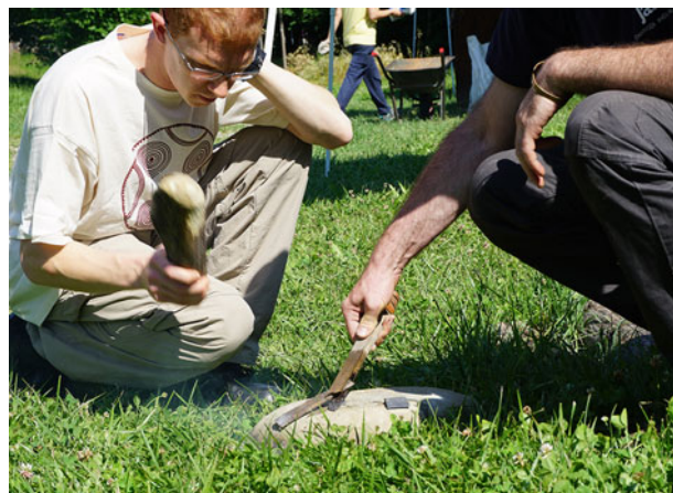
Fig. 1. Breaking a replica bronze sword using an antler hammer
