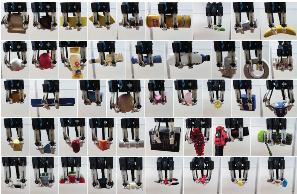
Figure 17. Examples of SAU-RFC hand grasping various objects from the YCB object set.
