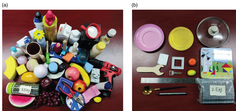
Figure 18. (a) Items from the YCB object set that the SAU-RFC hand was able to grasp in 10 times and (b) items from the YCB object set that the SAU-RFC hand was unable to grasp in 10 times.
