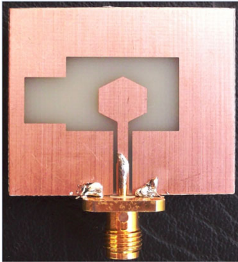
Fig. 2. Photograph of the fabricated antenna.
