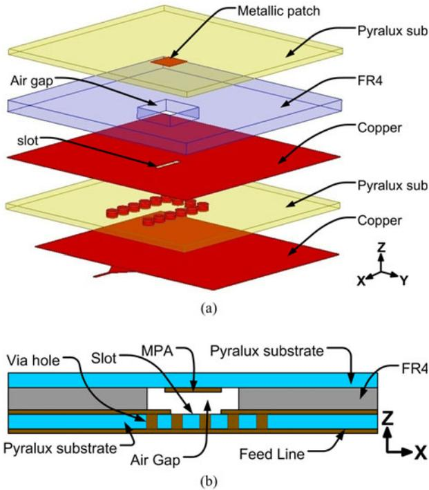
Fig. 1. Proposed membrane antenna geometry. (a) 3D layered model. (b) 2D side view.
