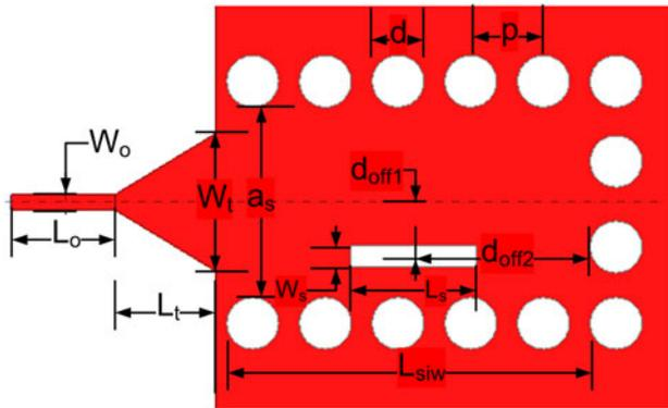
Fig. 2. Top view of SIW antenna along with rectangular slot.
