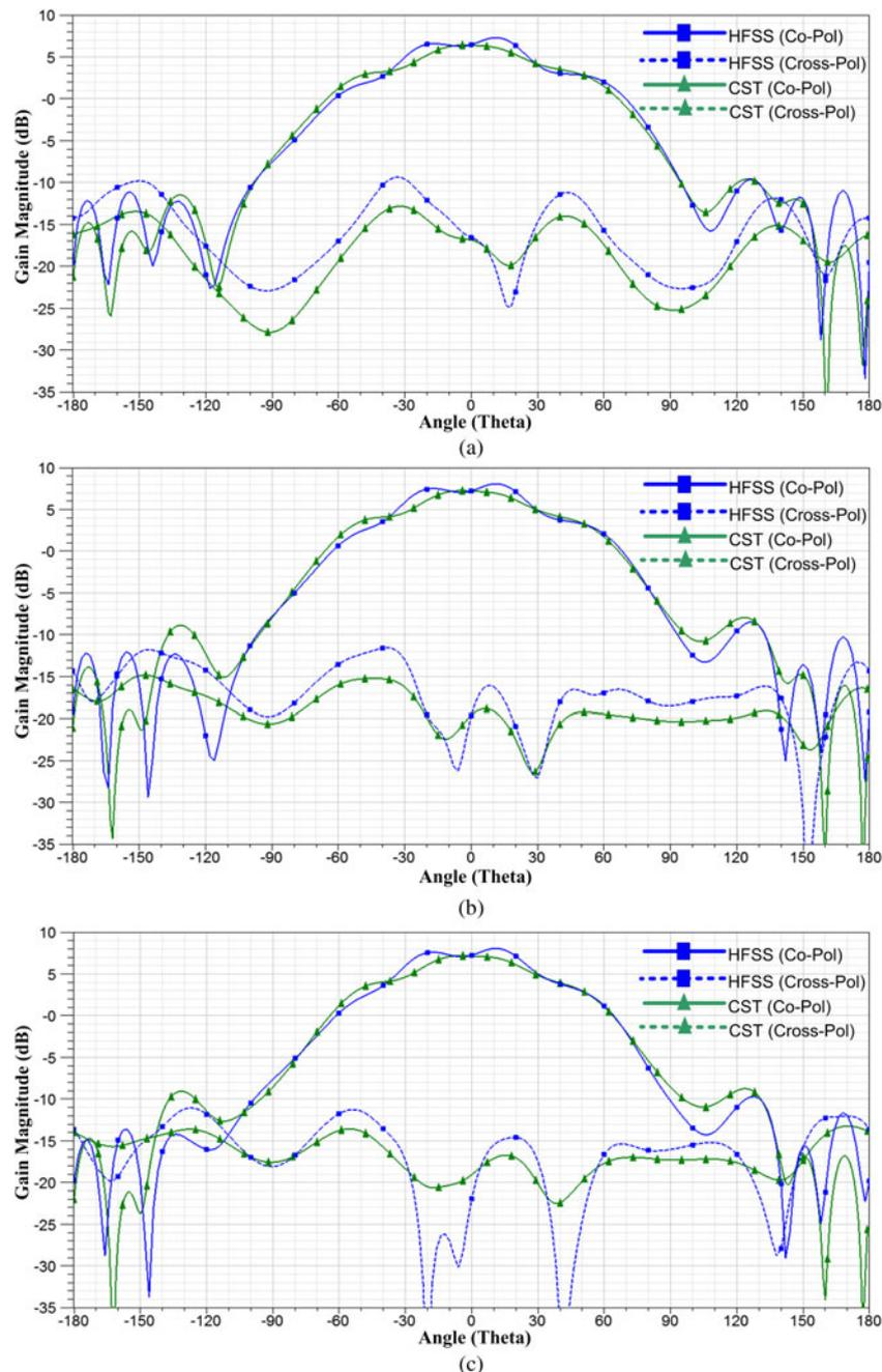
Fig. 6. 2D radiation pattern in  $E$ -plane with co- and cross-polarization. (a) 92 GHz. (b) 94 GHz. (c) 96 GHz.
