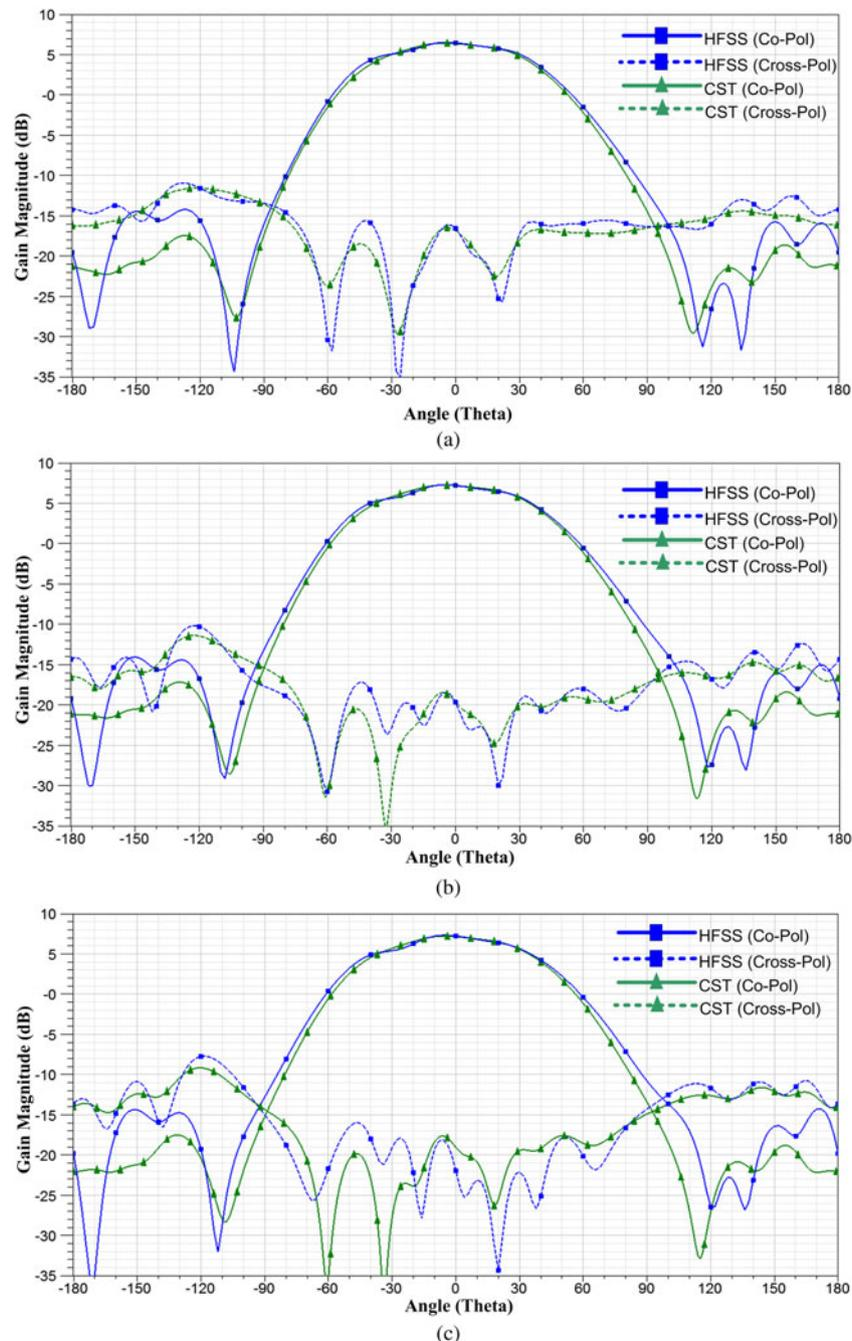
Fig. 5. 2D radiation pattern in  $H$ -plane with co- and cross-polarization. (a) 92 GHz. (b) 94 GHz. (c) 96 GHz.
