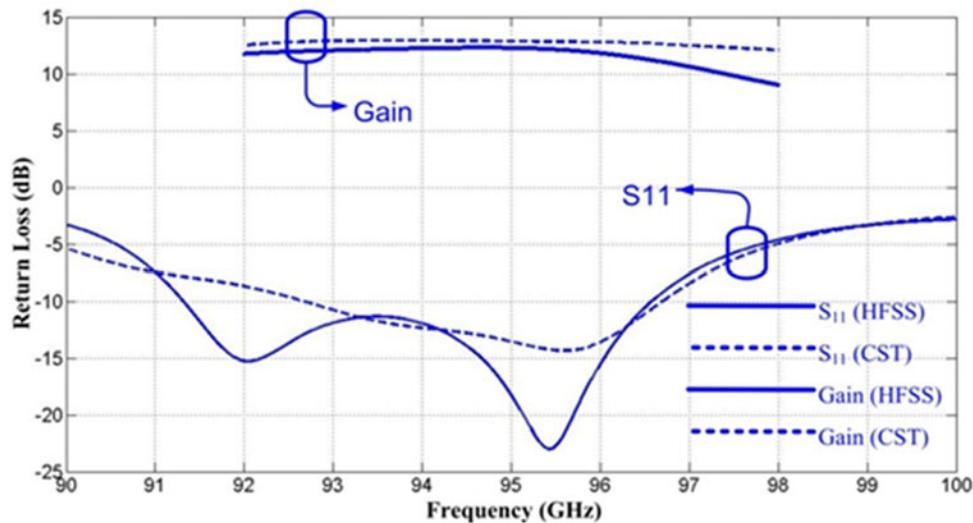
Fig. 10. Simulated return loss  $S_{11}$  and realized gain for  $1 \times 4$  array.
