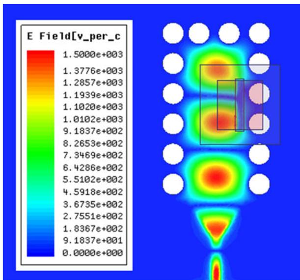
Fig. 8. Electric field distribution of the proposed single antenna.
