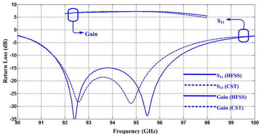
Fig. 4. Simulated return loss  $S_{11}$  and realized gain.
