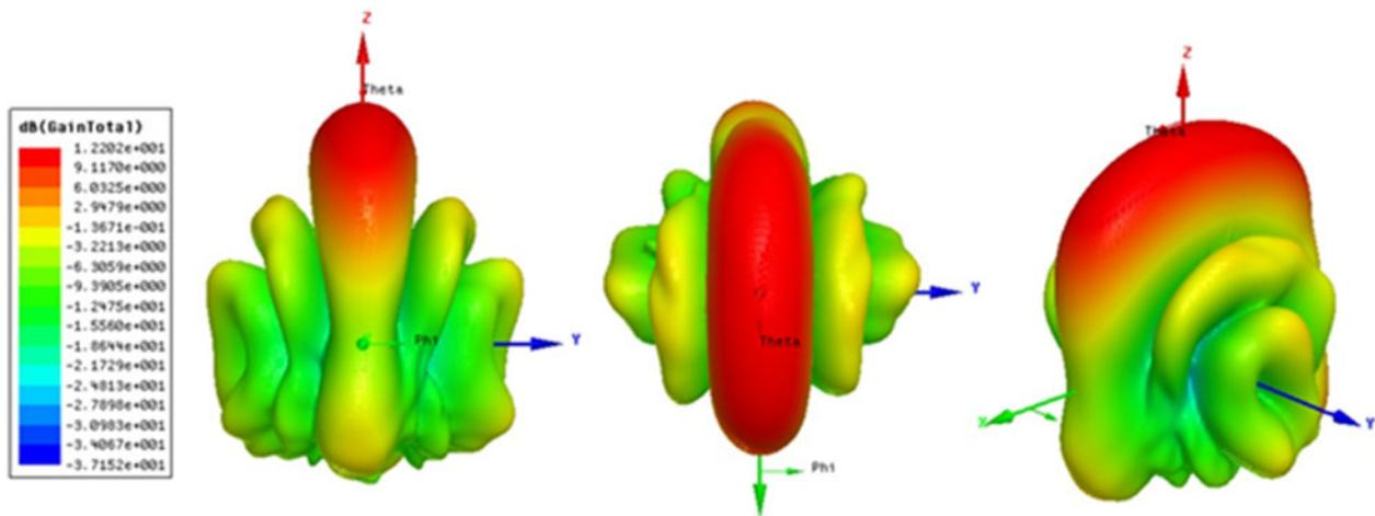
Fig. 12. 3D radiation pattern of proposed  $1 \times 4$  array.
