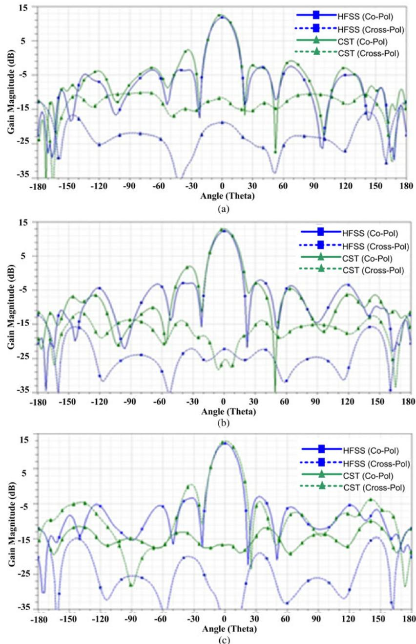
Fig. 11. 2D radiation pattern in  $E$ -plane with co- and cross-polarization. (a) 92 GHz. (b) 94 GHz. (c) 96 GHz.
