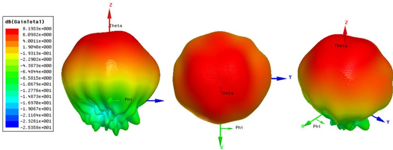
Fig. 7. 3D radiation pattern of the proposed single antenna.
