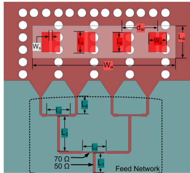
Fig. 9. Top view of proposed  $1 \times 4$  element array with,  $d_{ar} = 2.03$  mm,  $L_a = 1.85$  mm,  $W_a = 8.14$  mm,  $L_1 = 2$  mm,  $L_2 = 1.345$  mm,  $L_3 = 2$  mm, and  $L_4 = 1$  mm.
