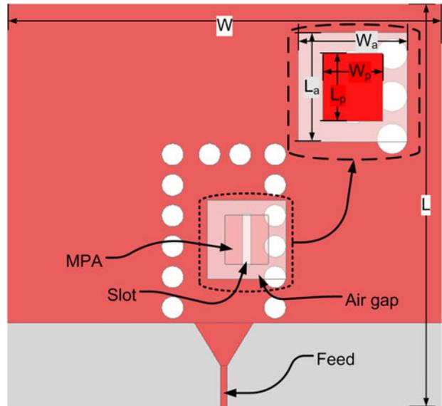
Fig. 3. Top view of proposed membrane antenna geometry.
