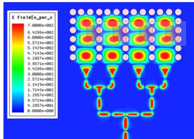
Fig. 13. The electric field distribution of the proposed  $1 \times 4$  array.
