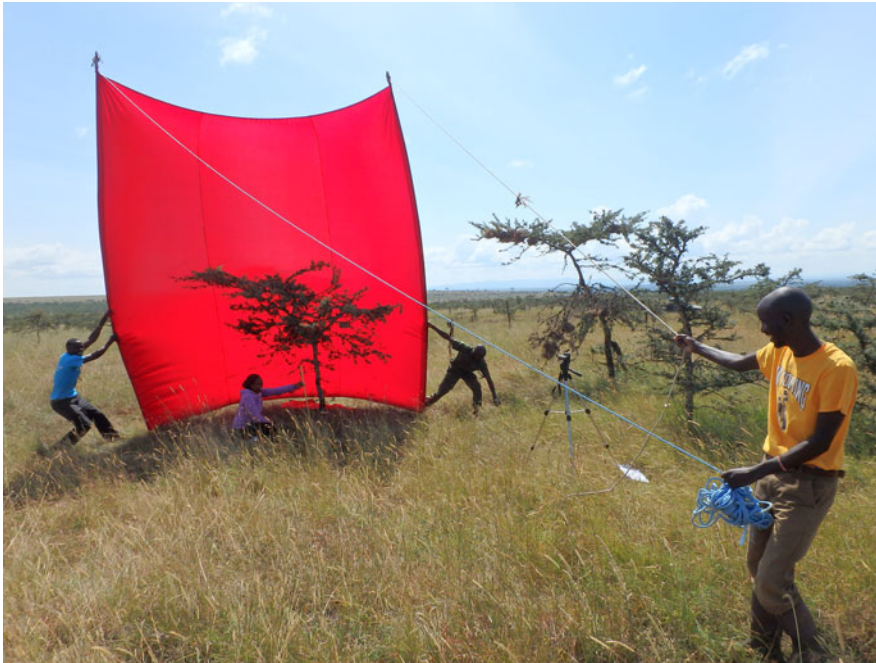
Figure 2. Photograph setup in the field, with camera situated 4 m from the target tree and oriented to 0°.
