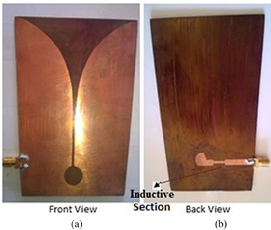
Fig. 12. Fabricated design of Vivaldi antenna (a) front view. (b) Back view showing feeder compensation (inductive section on feedline).
