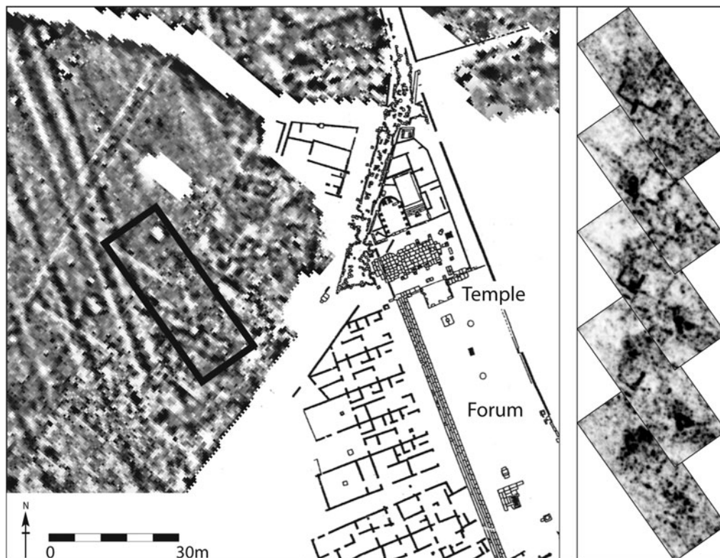
Fig. 2. Lucus Feroniae. Left : detail of the gradiometer survey results near the forum. The rectangle denotes the area of the GPR survey. Right : horizontal slices of the GPR survey results at increasing depths showing the changing nature of the buried remains.
