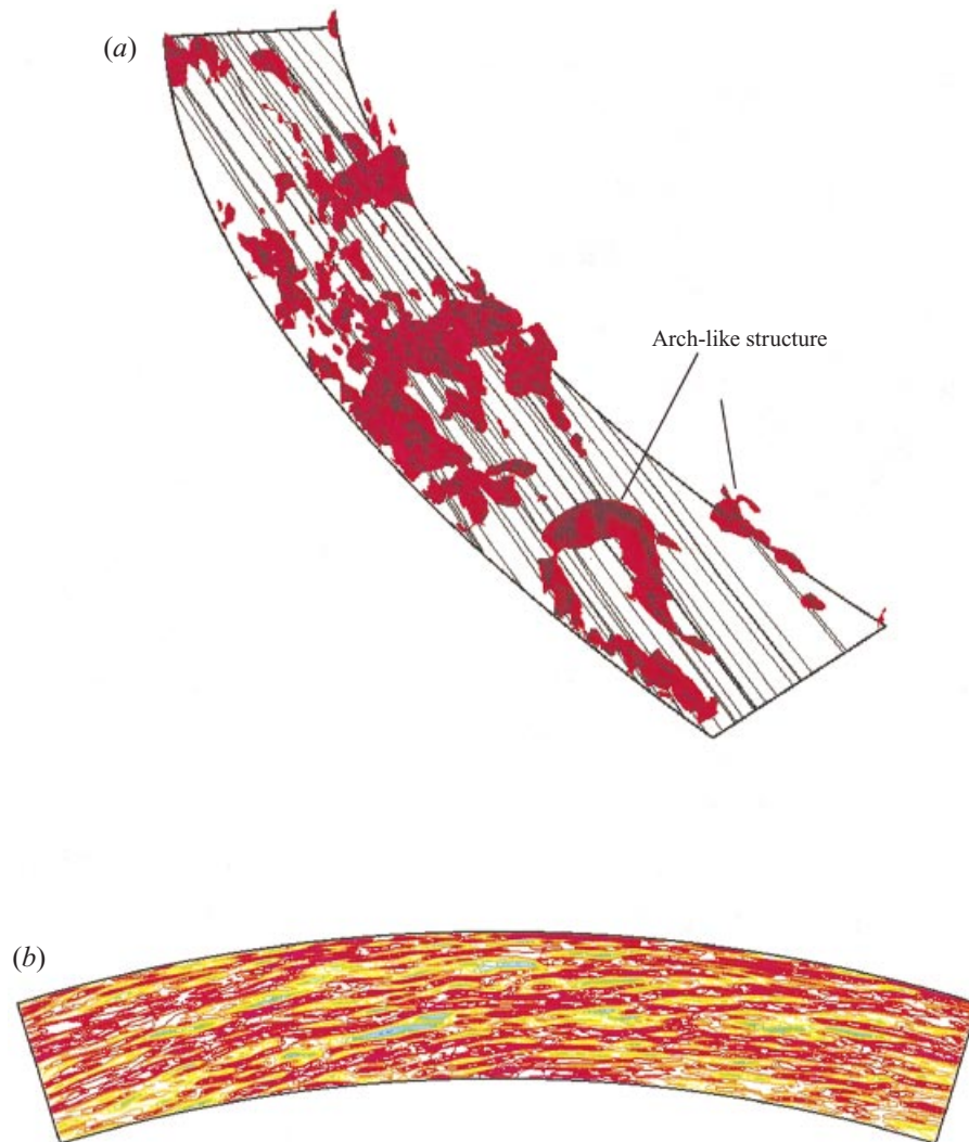
FIGURE 11. (a) Isosurfaces of instantaneous low-pressure cores showing the vortical structure similar to Robinson (1991), also shown are surface streamlines at the same instant; (b) instantaneous azimuthal velocity fluctuations \bar{v}'_{\theta}/\omega r at z^+ \approx 5 , contours vary from -0.68 to 0.32 , with an increment of 0.04 .
