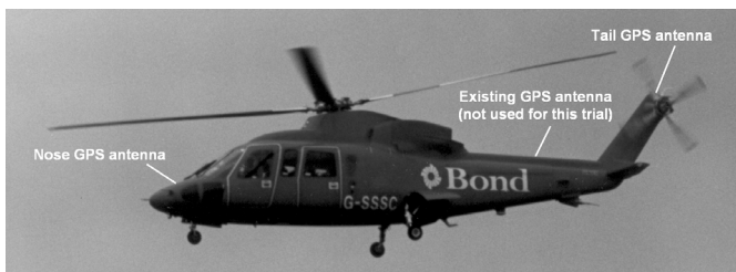
Figure 1. Sikorsky S76C trials airframe showing GPS antenna positions.
