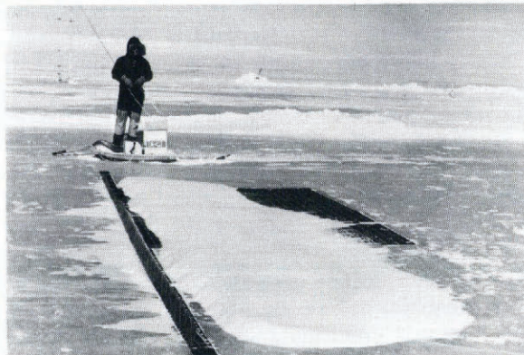
Fig. 1. 1/30 scale model snow fences on Diamond Lake, 30 January 1979. A portion of the 10 m wind-profile mast can be seen in the background.
