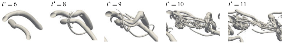
FIGURE 12. Description of the orthogonal reconnection event occurring for the case h/R=0.61 , r_c/h=0.166 and Re_\Gamma=7000 . Q -criterion iso-surfaces plotted in the region of interest at different times during the reconnection.
