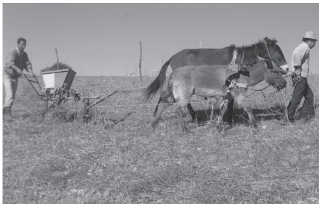
Figure 2. Seeding barley using an animal-drawn direct seeder in Sehoul, Morocco (photo by Mohamed Sfa).
