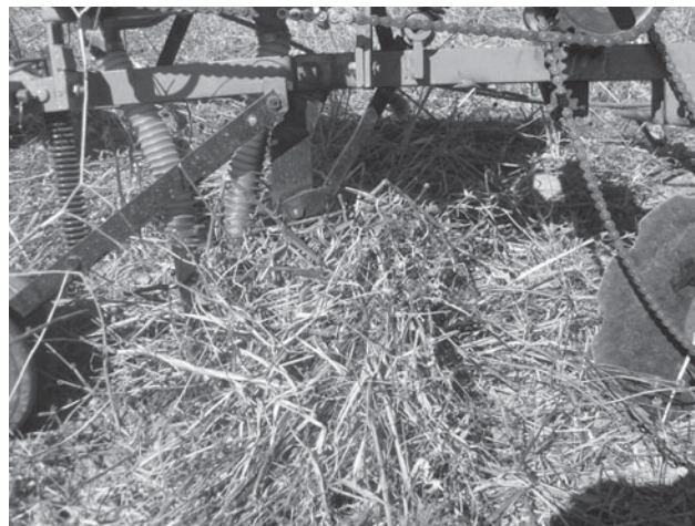
Figure 3. Straw accumulations beneath the direct seeder (photo by Mohamed Sfa).
