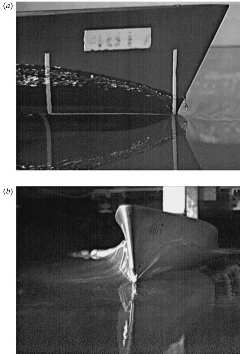
FIGURE 7. Two views of the laser sheet (film) around the bow of the ship model.
