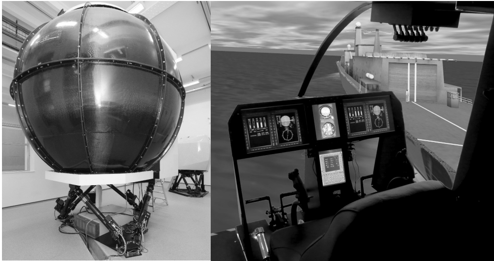
Figure 2. The HELIFLIGHT-R simulator; (a) Motion platform and display dome, (b) Pilot's view of the dynamic interface simulation and cockpit.
