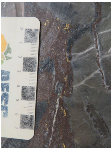
Fig. 3. Hand-specimen image of cut slice of ore from the Hera deposit showing abundant visible gold in sphalerite–galena (scale bar is in mm).
