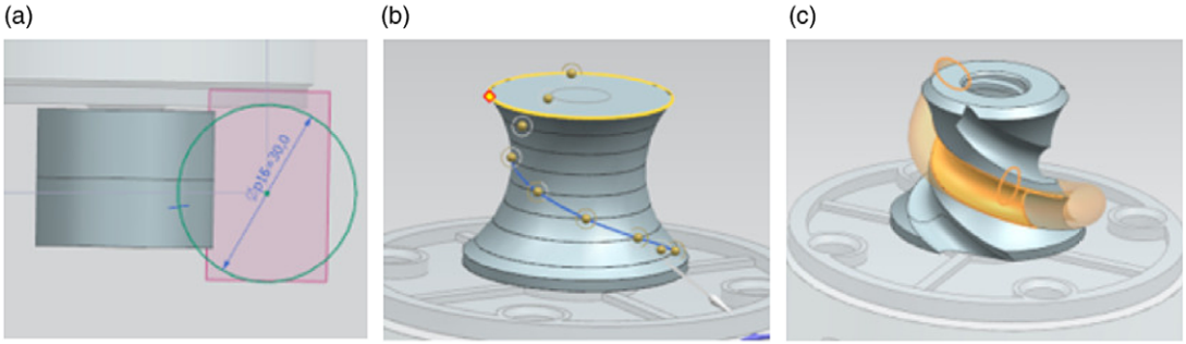
Figure 9. Graphic process of constructing a globoid, (a) sketch of a curved trajectory, (b) division of the globoids into parts of equal height, (c) creation of a curved surface.
