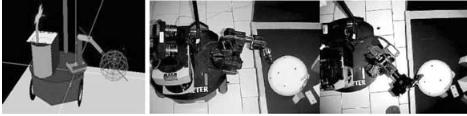
Fig. 21. (a) Simulation of the motion over a sphere. (b) and (c) Two of the images in the sequence of the real experiment.
