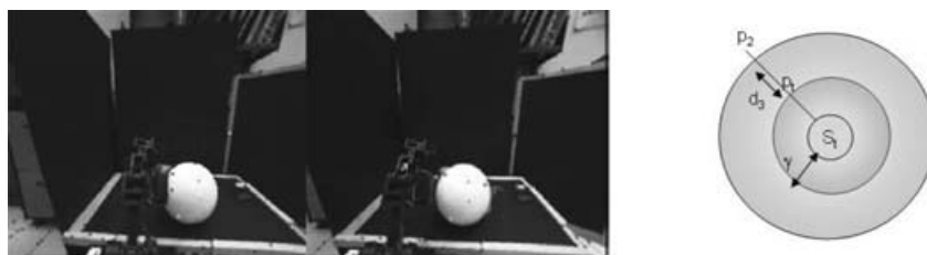
Fig. 20. (a) Points over the sphere as seen by the robot “Geometer”. (b) Guiding spheres for the arm’s motion.
