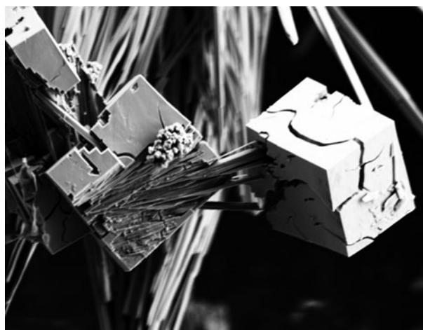
Fig. 2. SEM back-scattered electron image of galeaclolusite fibres protruding from fractured cubes of bariopharmacoalumite. Field of view: 20 \mu\text{m} . Photo Vincent Bourgoïn/Association Jean Wyart, Paris, Museums Victoria specimen M52929.
