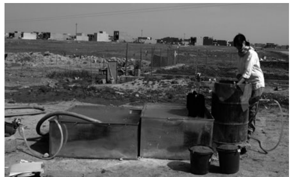
120. Example of a flotation machine designed for water recycling. © A. Livarda.
