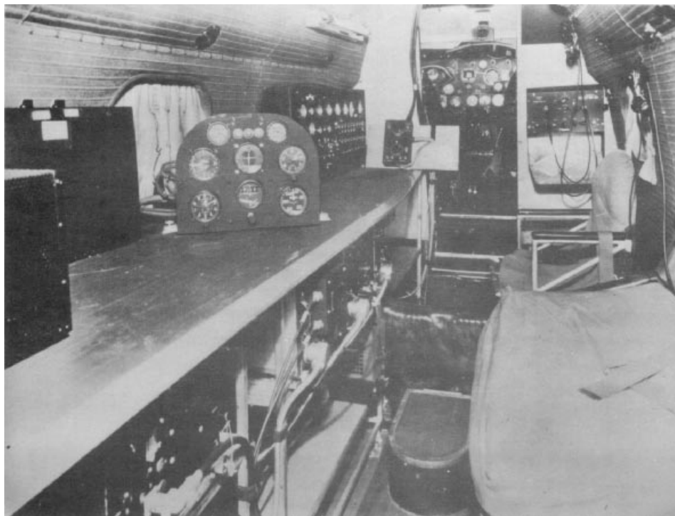
Figure 1. Interior view of NC-11 showing work bench replacing passenger seats on the left side. Test instruments and panel operator's seat are forward of the wing spar. Aft, on the bench, is an auxiliary set of instruments for the visitors who would be seated on the couch along the right side. During 1946, ILS and other navigation facilities under development at CAA Experimental Station, Indianapolis were demonstrated to delegates from the Provisional International Civil Aviation Organization. Roscoe Turner flew this Boeing 247-D in the 1934 London–Melbourne air race. In 1952 it was flown to Washington, retired permanently, repainted, and hung from a ceiling in the Smithsonian Museum.
