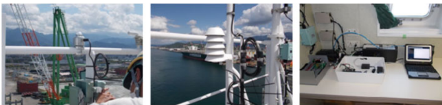
Figure 5. Photographs of the pyranometer (left), thermohygrometer (centre) outside the bridge and the devices for data storage inside the bridge (right).
