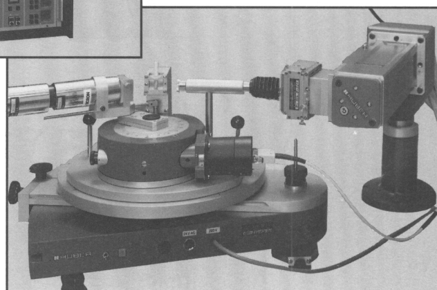
HUBER 653: For plane solid samples or thin films at room temperature.
