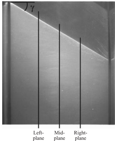
FIGURE 2. Plan view of the location of the three planes used for streak photography. The planes are at 30% (left), 50% (mid), and 70% (right) of the line spanning the test section.
