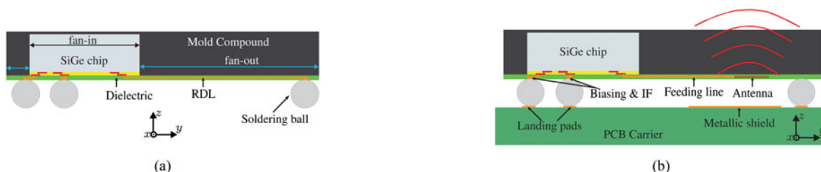
Fig. 1. SiP concept. (a) An embedded water level ball grid array (eWLB) package and (b) eWLB package and integrating an antenna and a chip.
