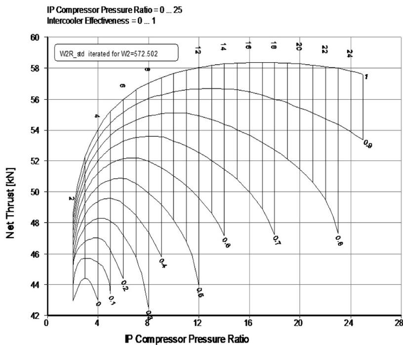
Figure 11. Plot of IPR and IC  $\epsilon$  vs net thrust for an aero engine with ICR core, fixed REC  $\epsilon$ , fixed pressure losses.
