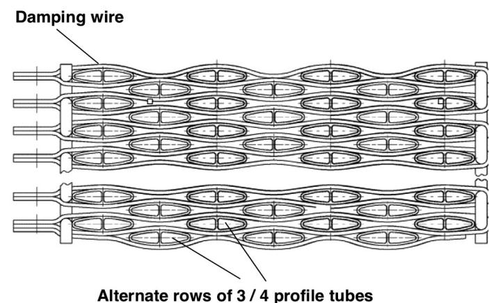
Figure 6. Details of the tubes in each recuperator module, as shown in Schoenenborn *et al* (2006).
