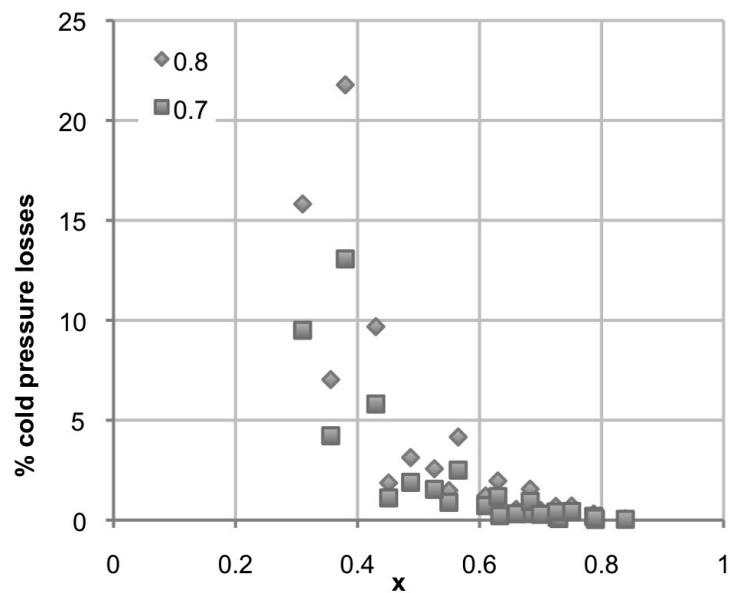
Figure 15. Chart showing values of optimum heat pipe parameter vs % intercooler cold pressure losses.
