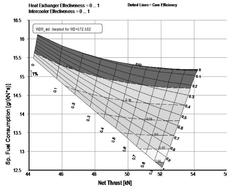
Figure 3. plot showing the relationship between net thrust, SFC and core efficiency for various intercooling and recuperative effectiveness. Simulation performed at fixed TET, BPR, pressure losses and at an optimum OPR.
