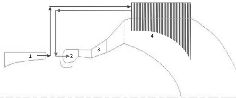
1 HPC, 2 Combustor, 3 Turbines, 4 HPHEX, 5 Nozzle
