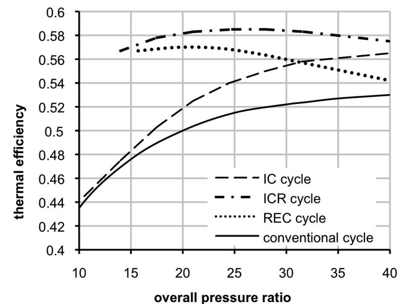
Figure 2. The comparison of the engine core efficiency for the simple cycle, intercooled, recuperated and intercooled-recuperated cycles for a number of OPRs and fixed TET.
