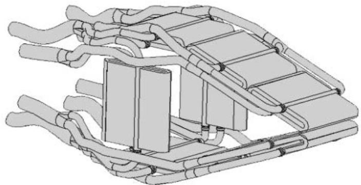
Figure 4. The recuperator design, as shown in Boggia *et al* (2005).
