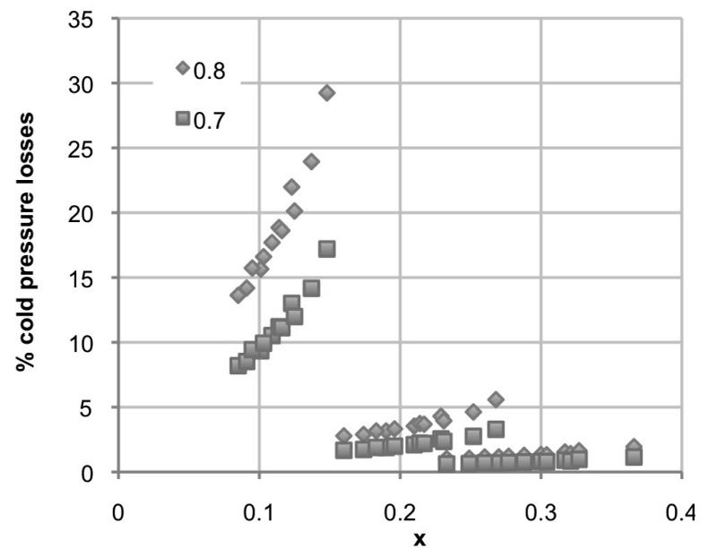
Figure 18. Chart showing values of optimum heat pipe parameter vs % recuperator cold pressure losses.
