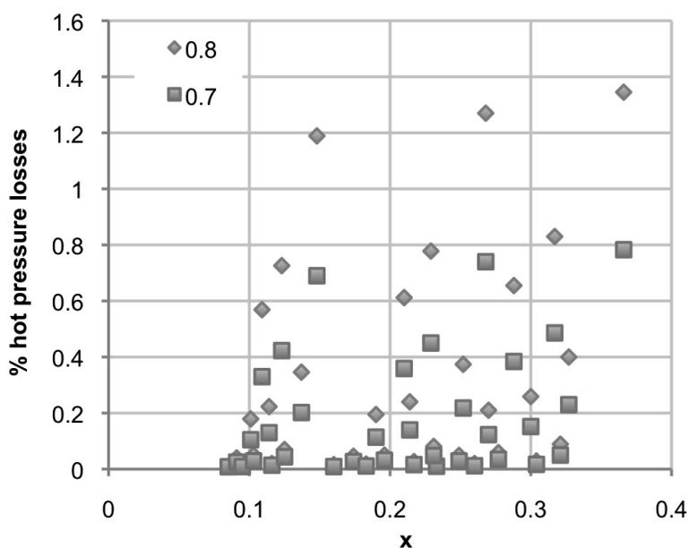
Figure 17. Chart showing values of optimum heat pipe parameter vs % recuperator hot pressure losses.
