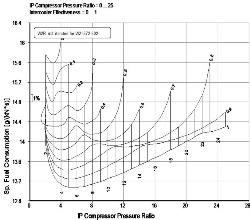
Figure 10. Plot of IPR and IC  $\epsilon$  vs SFC for an aero engine with ICR core, fixed REC  $\epsilon$ , fixed pressure losses.
