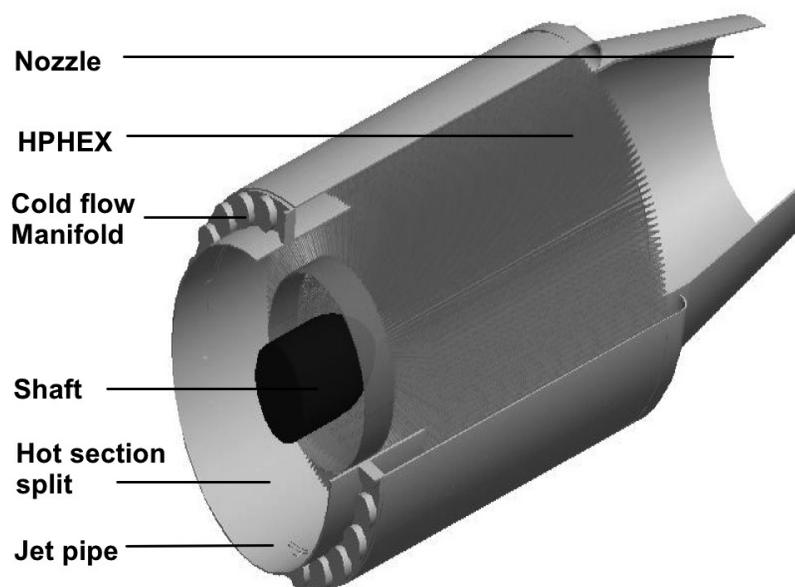
Figure 8. Schematic showing how the HPHEX protrudes from the jet pipe to the cold flow jacket.
