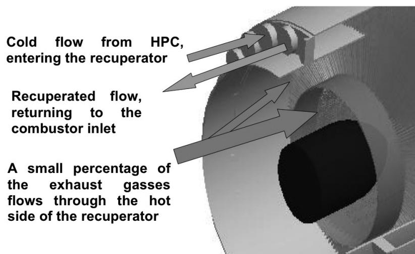
Figure 9. Details of the flows in the HPHEX.
