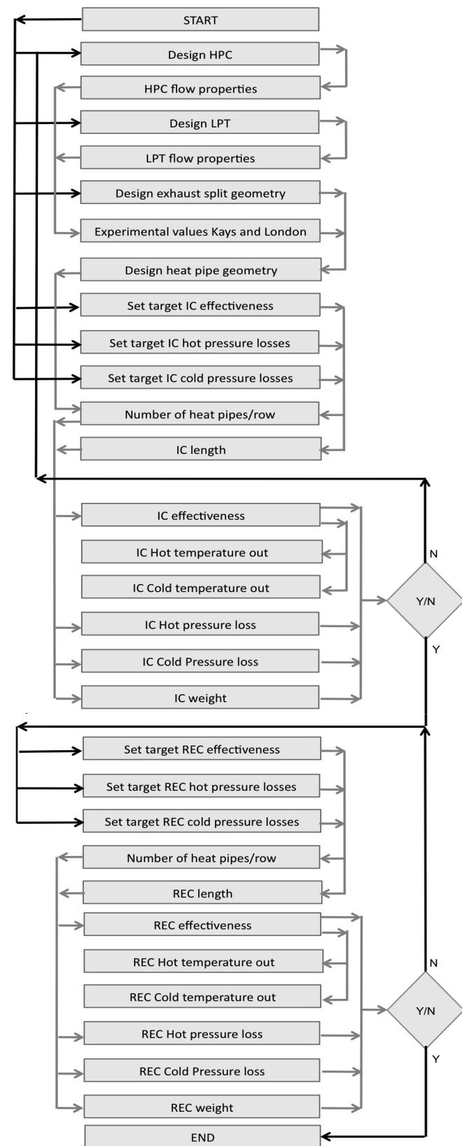
Figure 12. The process flow chart for the HPHEX design software as applied to the ICR aero engine.
