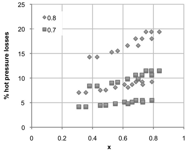
Figure 14. Chart showing values of optimum heat pipe parameter vs % intercooler hot pressure losses.
