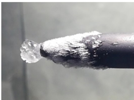
Figure 2. Iced pressure port of the AN5815 Pitot probe.
