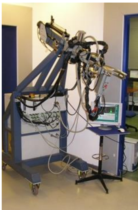
Figure2. DifRob ® , the prototype for on site XRD measurements developed by XRD-Tools
