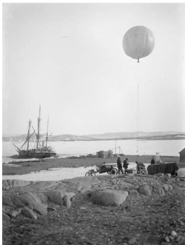
Fig. 4. Mylius-Erichsen equipped the expedition with an automobile, intended for crossing frozen fjords. This did not work, and the axle was used as a winch to operate weather balloons.
