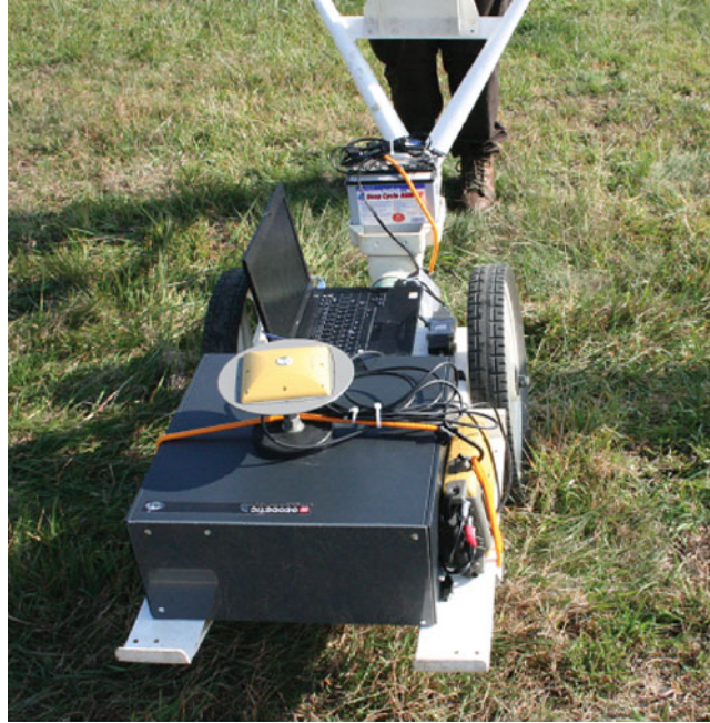
Figure 2. The NRL cart-based system with OSU's dual-IMU/GPS geolocation system.
