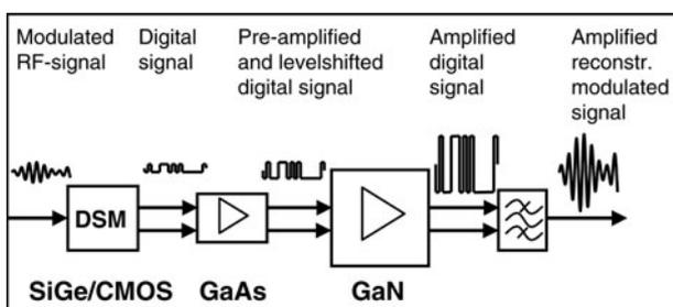
Fig. 7. Architecture of class S amplifier.
