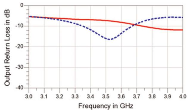
Fig. 3. Output return loss of class AB amplifier (simulation (dotted) versus measurements (solid)).
