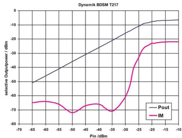
Fig. 11. Dynamic range of this 450 MHz BDSM: signal power and intermodulation distortion of BDSM bit sequence as a function of modulator input power.
