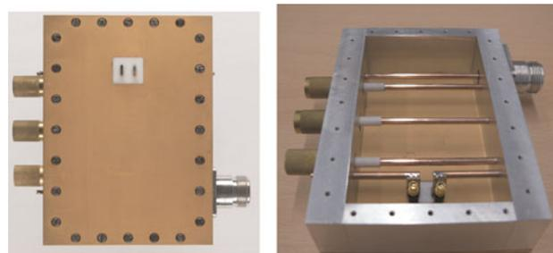
Fig. 14. Photographs of the reconstruction filter in comb line filter technology. Left: view on filter top side with balanced input pins fixed by a PTFE feed through, right: view on filter inside with bottom cover removed.
