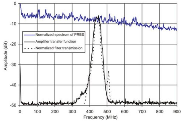
Fig. 16. Characterization of amplifier transfer function (solid black curve), for comparison: spectrum of PRBS (solid gray curve) and filter transmission (dashed curve).
