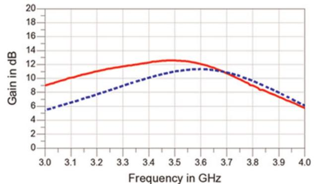
Fig. 4. Small-signal gain of class AB amplifier (simulation (dotted) versus measurements (solid)).
