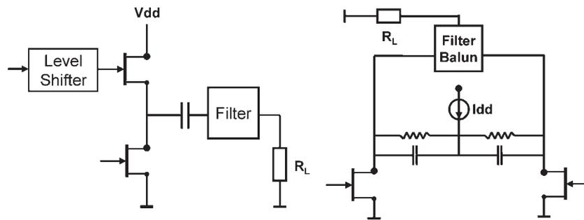
Fig. 8. Principal schematic for voltage switched amplifier (left) and current switched amplifier (right).
