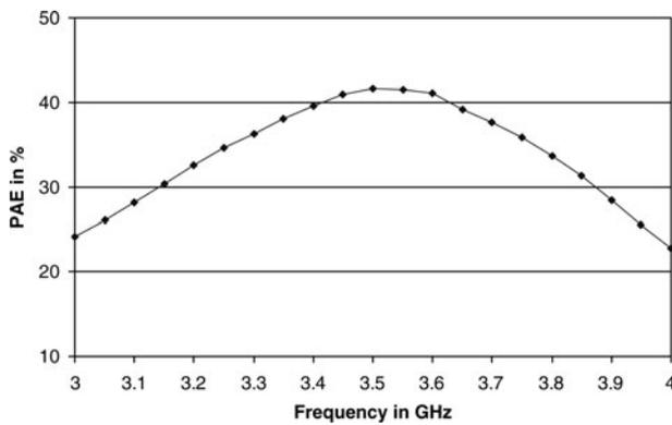
Fig. 6. PAE of class AB amplifier at 35 dBm input power.
