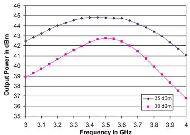
Fig. 5. Output power of class AB amplifier at 35 dBm input power.
