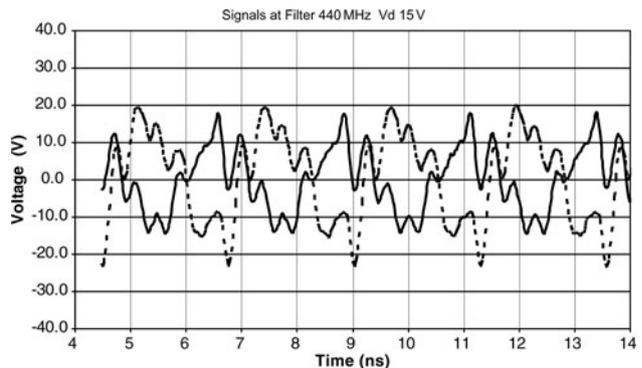
Fig. 17. Time domain signals at filter input pins (drain voltage 15 V).
