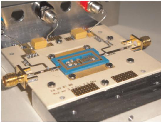
Fig. 1. Class AB amplifier for WiMAX operation.
