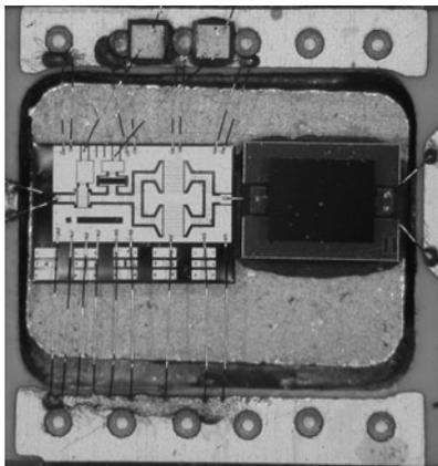
Fig. 13. Photograph of the mounted GaN MMIC and GaAs diode.
