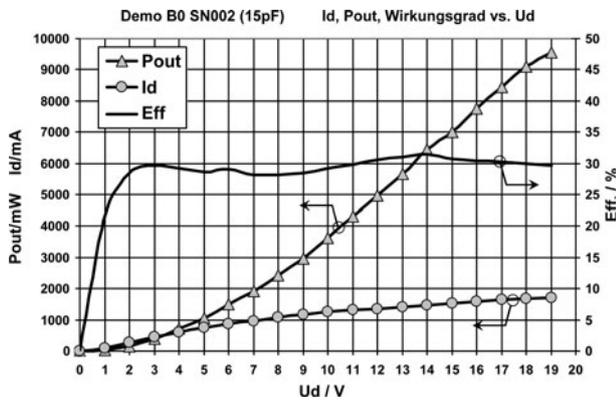
Fig. 18. Drain efficiency, output power, and drain current versus supply voltage.
