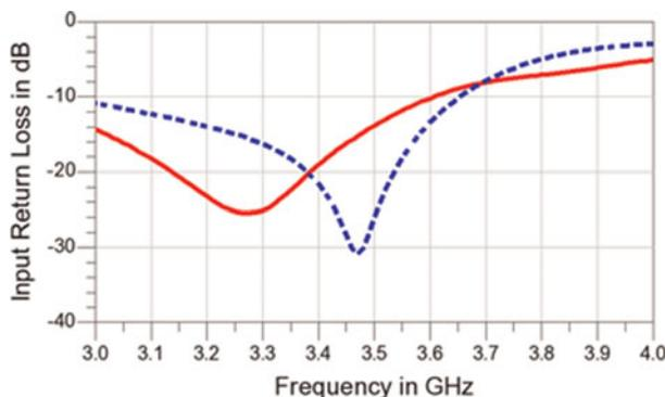
Fig. 2. Input return loss of class AB amplifier (simulation (dotted) versus measurements (solid)).
