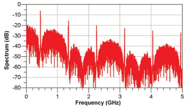
Fig. 10. Wide-band spectrum of a BDSM signal.
