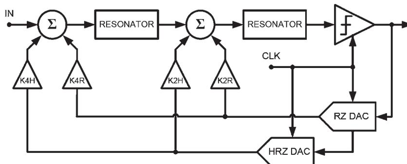
Fig. 9. Block diagram of fourth-order bandpass DSM.
