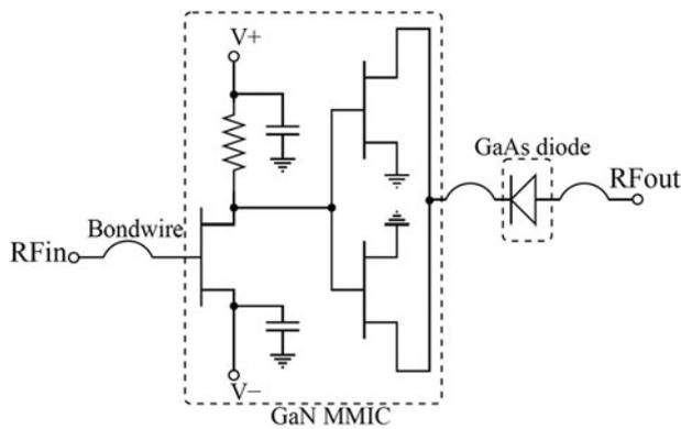
Fig. 12. Schematic of the switch mode amplifier configuration.
