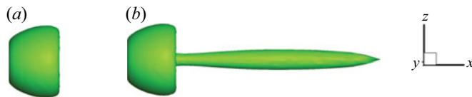
Figure 8. Isosurfaces of Q = 0.01 for the streamwise rotating circular disk at Re_s = 100 with different Reynolds numbers of rotation: (a) Re_r = 50 , (b) Re_r = 100 .
