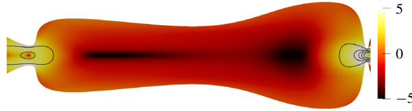
FIGURE 5. (Colour online) Spatial distribution of the absolute value of the decay rate production in the optimized channel (on a logarithmic scale), \ln(-\sigma_\Omega) . Black lines correspond to the oscillating flow velocity magnitude isolines \hat{u} = \text{const} .
