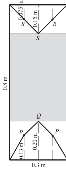
FIGURE 6. Split of the oscillating water tunnel cross-section between areas of influence of the sidewall, top and bottom boundary layers (thick solid lines), by matching velocities at points P , Q , R and S . The shaded area corresponds to the main sidewall region, with a flux per unit height of q_{sw} . The specific dimensions indicated in the figure correspond to application of our model to test 1 reported by Ribberink & Al-Salem (1995), assuming the top boundary to be smooth.
