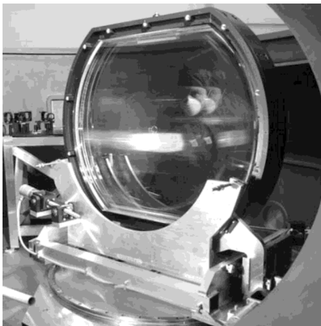
Fig. 2. The 940 mm diameter gold coated diffraction gratings used in the pulse compression during an optical inspection.
