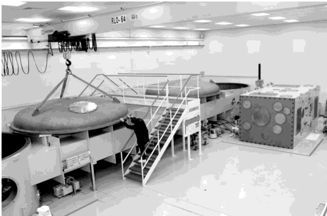
Fig. 7. The petawatt Facility prior to the installation of the target chamber radiation shielding.
